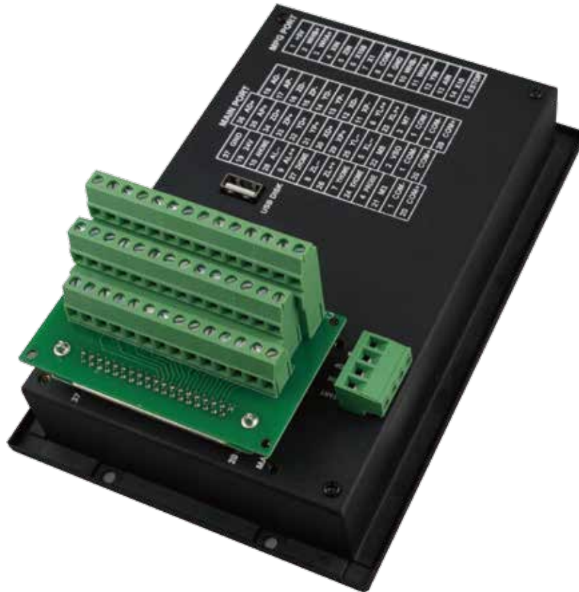
Picture 2-8 Main Port with wiring terminal
